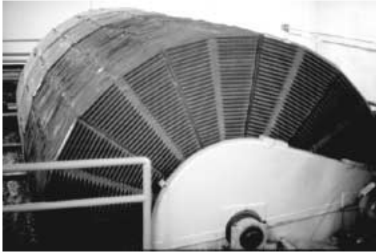
Figure 8-45(b) Aerobic fixed film systems; rotating biological contactor (RBC). (Photo courtesy of U.S. Filter/Envirex.)
