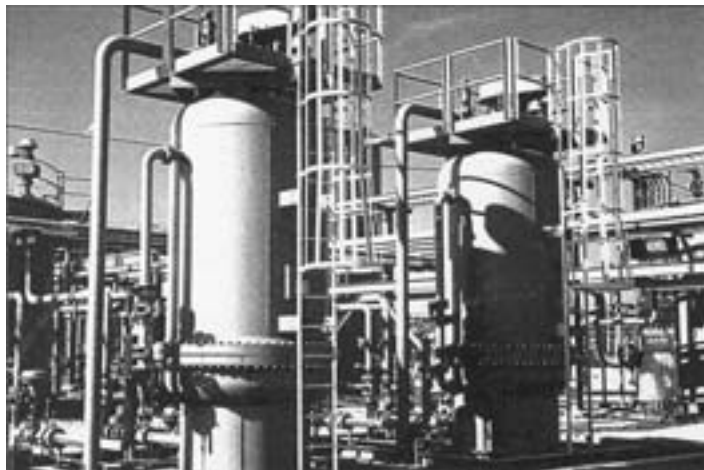
Figures 8-73(e) Pressure and vacuum filters. (Courtesy of EIMCO Process Equipment, a Baker Hughes Company.)
