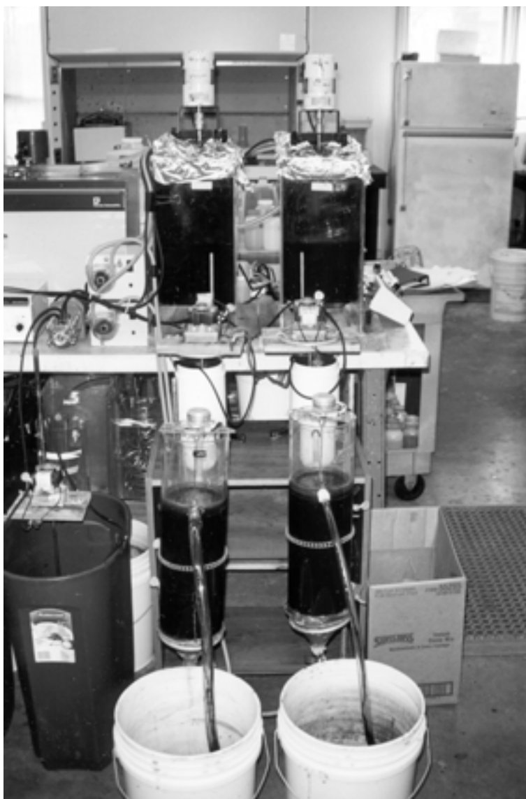
Figure 1-3(d) Photograph of a block aerator set-up for performing treatability studies in the laboratory. (Courtesy of AWARE Environmental, Inc.)
