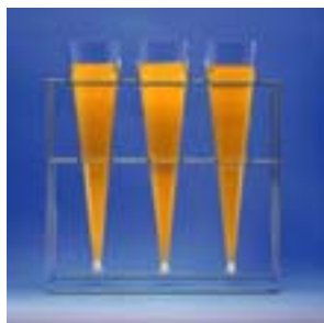
Figure 6-6 Imhoff cones used to measure settleable solids. (Courtesy of Wheaton Science Products.)
