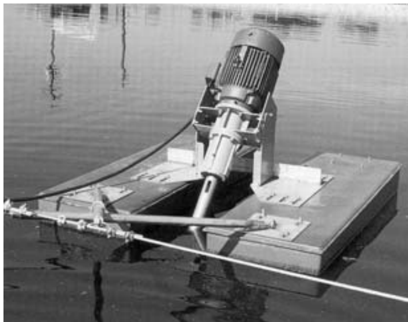
Figure 8-38(k) Alternative device for aeration: Pontoon-mounted, aspirating aerators. (Photo courtesy of Eimco Process Equipment, a Baker Hughes company.)
