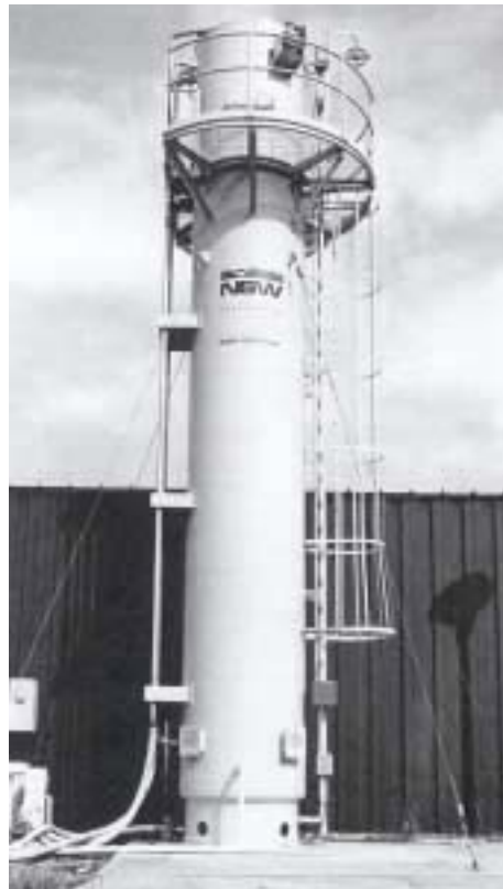
Figure 8-45(c) Aerobic fixed film systems; fluidized bed. (Photo courtesy of NSW Corporation.)
