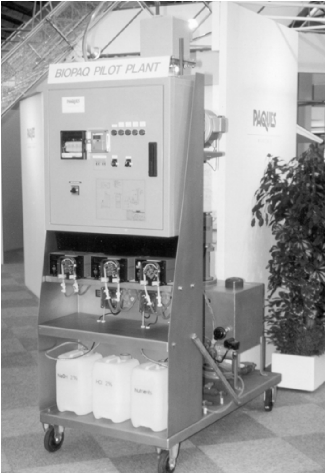
Figure 1-4 Photograph of a pilot scale wastewater treatment system. (Courtesy of Paques ADI, Inc.)
