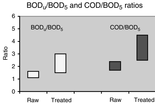
Figure 2.12. Ranges of values of the ratios BOD u /BOD 5 and COD/BOD 5 for raw sewage and biologically treated sewage
